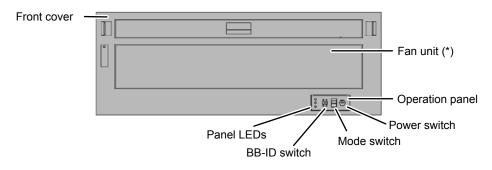
\*: You can see the fan unit by removing the front cover.
